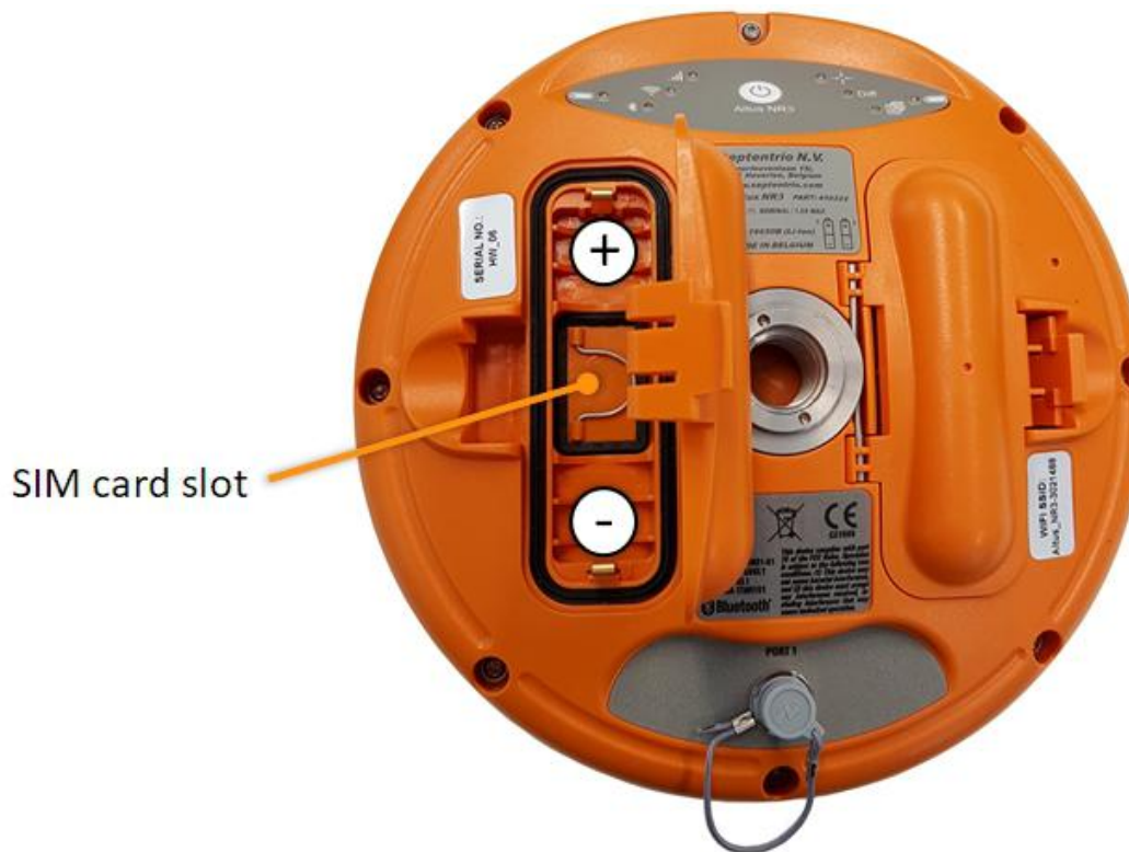
Figure 2-3: Underside of the Altus NR3 indicating the location of the SIM card slot
