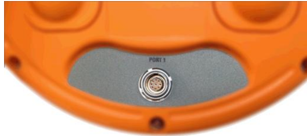
Figure 2-5: Altus NR3 Port 1 Connection
